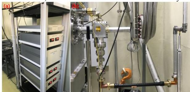
Figure 4: RF test of a HWR cryomodule. (a) SSPA and (b) the connection of a coaxial line to a power coupler in the cryomodule.
