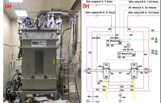
Figure 3: Picture of (a) the HWR cryomodule in horizontal test facility and (b) the P&ID for the HWR cryomodule.
