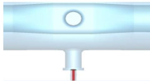
Figure 7: A modified design of electrically coupled antenna.
