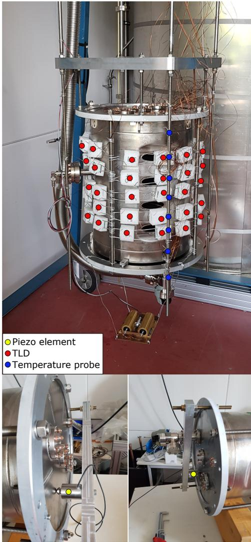
Figure 2: Vertical string with cavity in a support frame equipped with TLD's, temperature probes and piezo elements.
