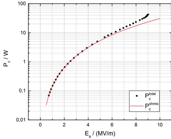
Figure 4: Total losses  $P_c^{total}$  as well as pure ohmic losses  $P_c^{ohmic}$  inside the cavity depending on  $E_a$ .
