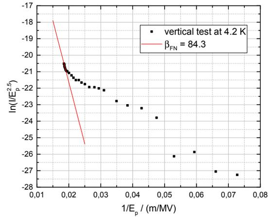
Figure 6: Fowler-Nordheim plot for the first RF test at 4.2 K.
