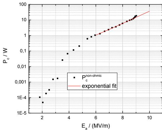
Figure 5: Non-ohmic losses  $P_c^{non-ohmic}$  inside the cavity depending on  $E_a$ .
