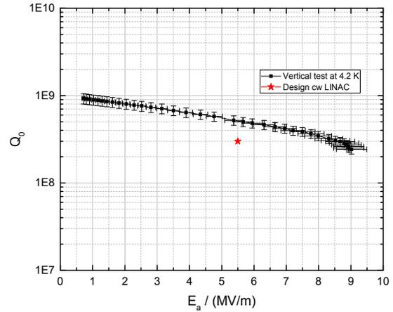
Figure 3:  $Q_0$  vs.  $E_a$  curve at 4.2 K.
