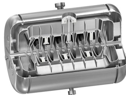
Figure 2: 3D model of the sc 217 MHz CH cavity [7].
