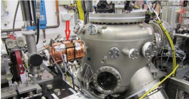
Figure 5: Cavity mounted at the REGAE beam line.
