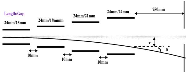
Figure 2: The 2D design of chopping cum deflecting system for HCL.
