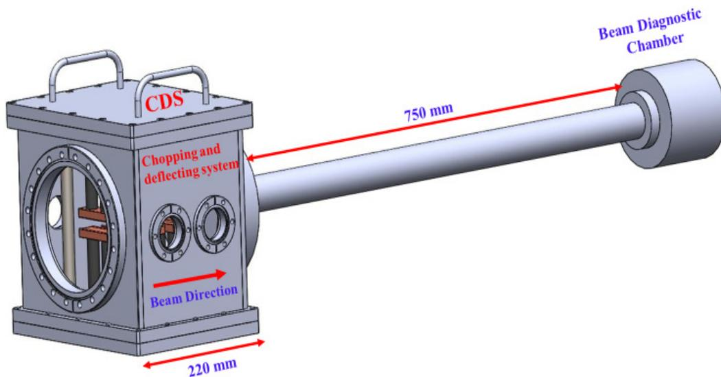
Figure 5: The CDS system including inner assembly, an outer chamber, the drift of length 750 mm, and a diagnostic box.
