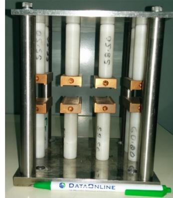
Figure 4: The complete inner assembly with its four pairs of deflecting plates.
