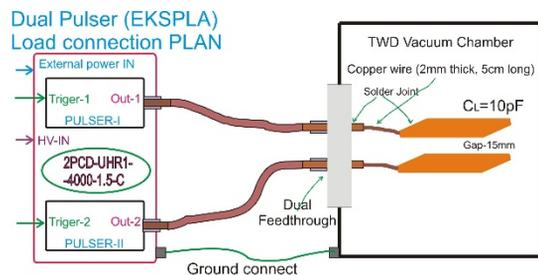
Figure 6: The deflector plates are connected to the power supply using feedthroughs. Results and Discussions.
