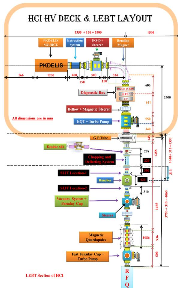
Figure 1: The location of CDS has been depicted in the layout of the LEBT section of the High Current Injector.
