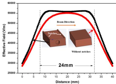
Figure 3: The plate design modification to improve the linearity and effective electric field.
