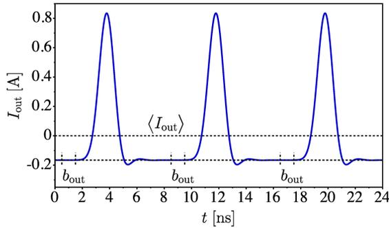
Figure 2: Drooped CT output signal for a CW input beam.
