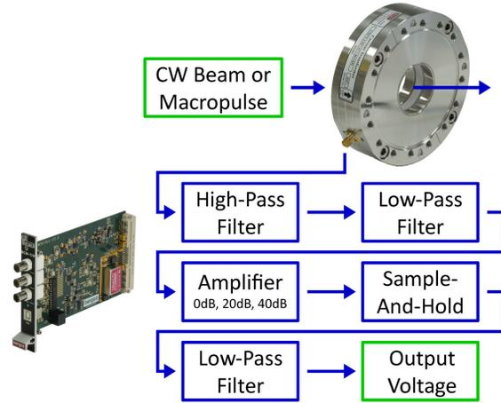
Figure 3: CWCT and BCM-CW-E principle.
