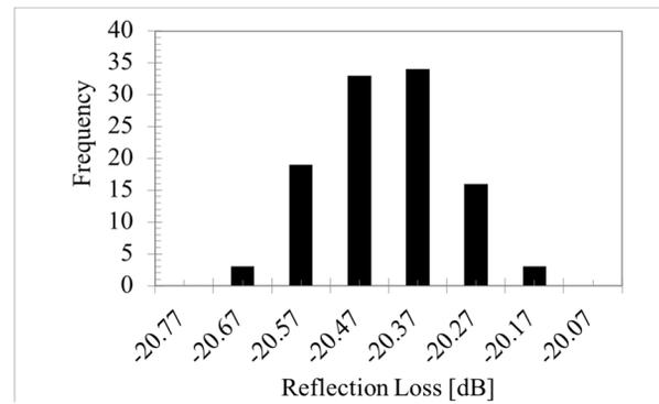
Figure 5: Reflection-loss values distribution of the 108 input ports of the rf power combiner. These values were measured by S21. The average reflection loss and its STD value are -20.469 dB and 0.105 dB, respectively.
