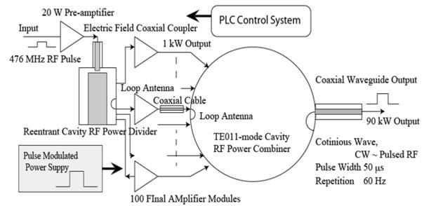
Figure 1: Block-diagram of the amplifier.
