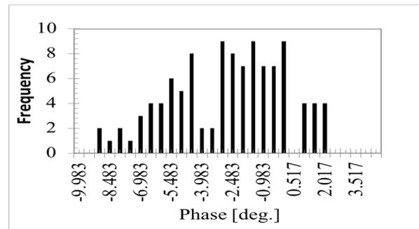
Figure 6: The phase deviation values distribution from the ideal at the 108 input ports of the rf power combiner. These values were measured by S21.
