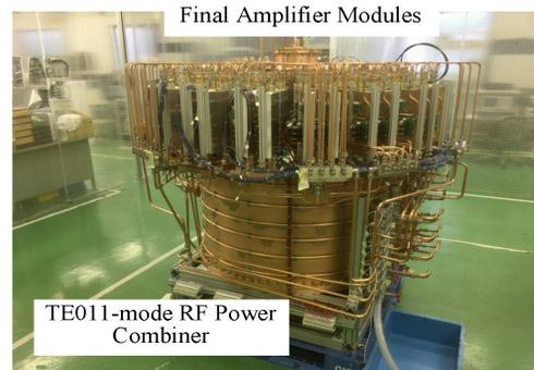
Figure 2: Actual fabrication condition of the amplifier.
