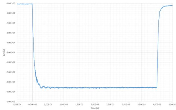
Figure 6: High Voltage Pulse Measured at 100 kW.
