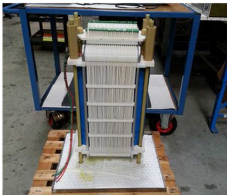
Figure 4: Pulse Transformer.
