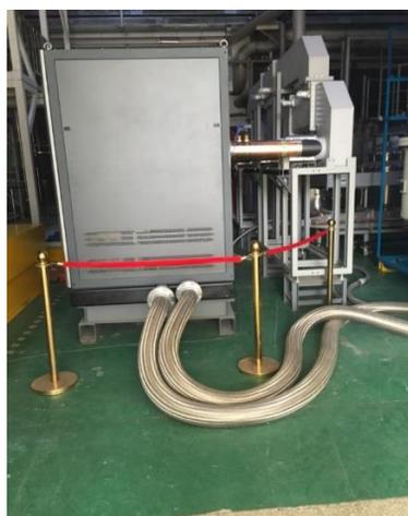
Figure 3: 650 MHz/150 kW SSA.
