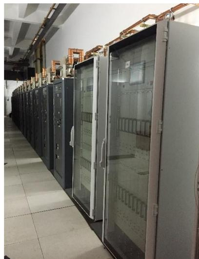
Figure 1: 325 MHz/10 kW SSA.
