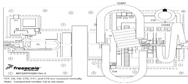
Figure 6: Reference circuit component layout.
