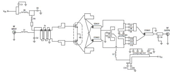
Figure 5: Reference circuit schematic.
