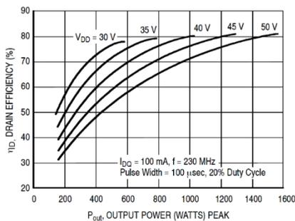
Figure 3: Drain Efficiency versus Output Power.
