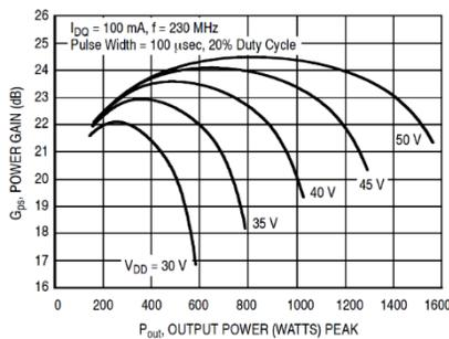
Figure 2: Power Gain versus Output Power Peak.
