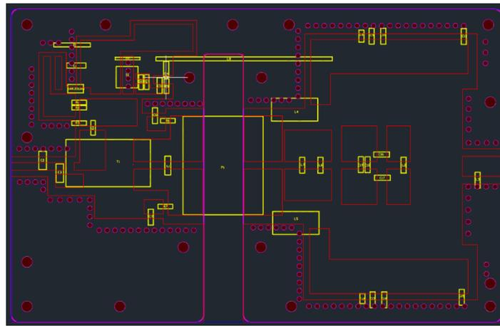
Figure 7: Amplifier module circuit component layout.
