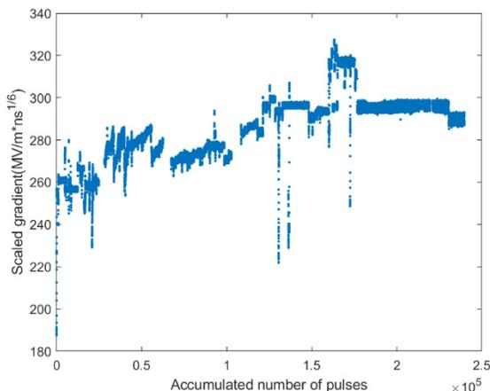
Figure 3: Scaled gradient vs number of accumulated pulses.
