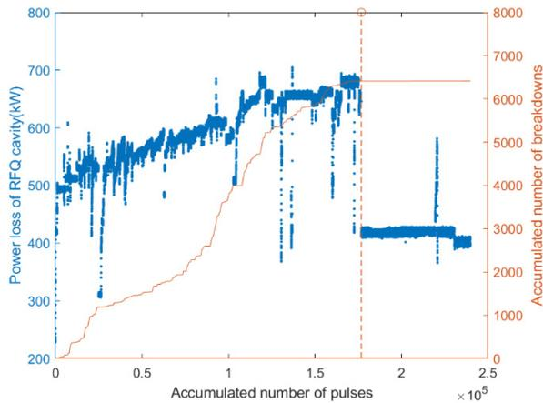
Figure 2: The blue dots represent power loss of RFQ, the red line represents accumulated number of breakdowns.
