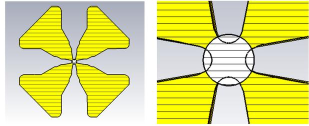
Figure 9: RFQ electrodes model.
