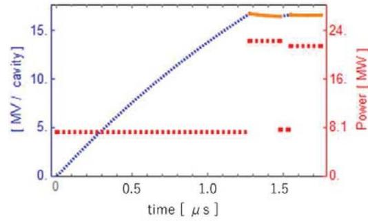
Figure 3: Accelerating voltage and RF power evolution of the L-Band TW accelerator by the quasi-perfect compensation are shown with the same manner in Fig. 3. The average acceleration voltage was  $16.60 \pm 0.14$  MV (peak-to-peak).
