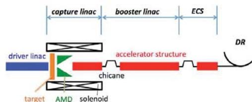
Figure 1: Schematic view of ILC E-driven Positron source.
