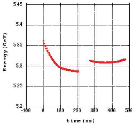
Figure 5: Expected energy after the booster for the macro-pulse. The horizontal axis is time in the macro-pulse.
