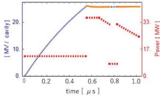
Figure 4: Accelerating voltage and RF power evolution of the S-Band TW accelerator by the quasi-perfect compensation are shown with the same manner in Fig. 3. The average acceleration voltage was  $25.76 \pm 0.19$  MV, (peak-to-peak).
