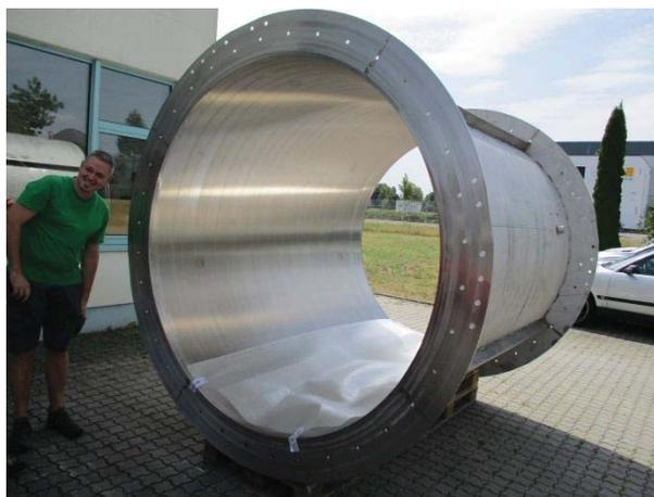
Figure 10: Dummy cavity ( $L=2.5\text{m}$ ,  $D_{\text{out}}=2.4\text{m}$ ) at the factory acceptance test (FAT).
