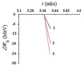
Figure 4: Losses of beam energy for different beam currents: 1 -  $I_b=1$  A, 2 -  $I_b=2$  A, 3 -  $I_b=3$  A.
