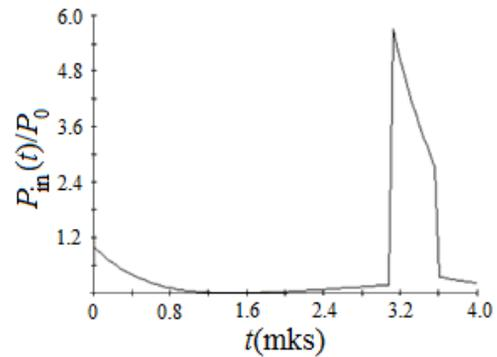
Figure 3: The envelope of RF power coming to input of the accelerating structure after the SLED system.
