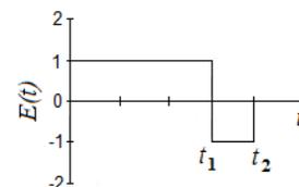
Figure 1: The RF power signal coming at the input of SLED system.
