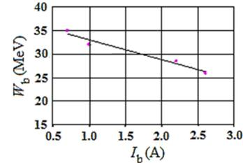
Figure 6: Position of the maximum of the energy spectrum depending on the current of the beam accelerated in one accelerating section of LUE-200 linac. Duration of the beam current is  $\tau_b = 0.1$  mks.
