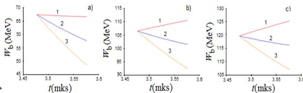
Figure 5: Full energies received by a beam in the accelerating structure for different RF power of the generator and different beam currents: a - TH2129 + SLED, b - E3730A + SLED, c - 5045 SLAC + SLED, 1 -  $I_b = 1$  A, 2 -  $I_b = 2$  A, 3 -  $I_b = 3$  A.
