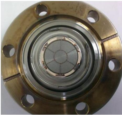
Figure 1: The EIMAC Y824 Cathode grid assembly.
