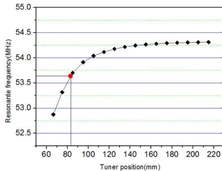
Figure 6: Frequency range of the DTL2 as a function of tuner position.
