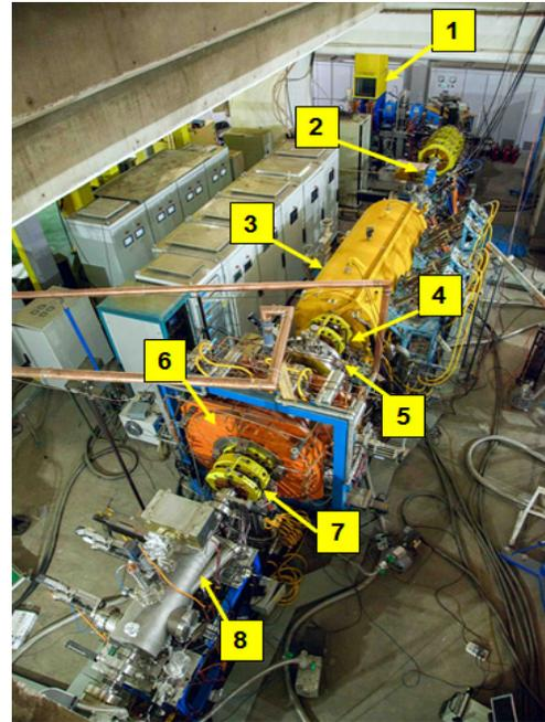
Figure 1: General view of the SSC-Linac. 1-ECR ion source; 2-LEBT section; 3-RFQ; 4-MEBT section; 5- Re-buncher cavity; 6- IH-DTL1; 7-Focusing triplets; 8-Beam diagnostics system.
