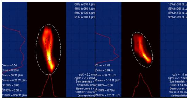
Figure 2: Measured transverse emittances after analysing dipole magnet.
