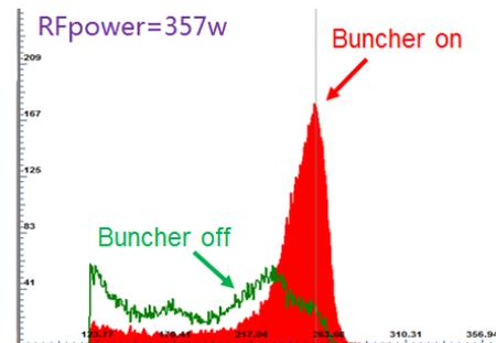
Figure 4: Measured bunch efficiency.
