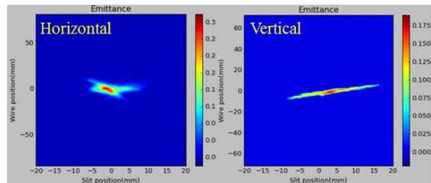
Figure 8: Measured transverse emittances at DTL1 exit.
