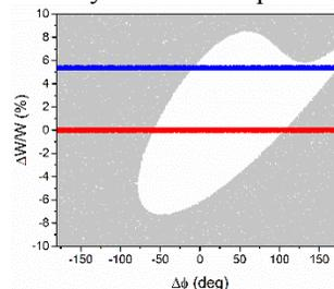
Figure 12: Simulated RFQ longitudinal acceptance and DC beam longitudinal distributions with input energy of 14 keV/u (red) and 14.75 keV/u (blue).
