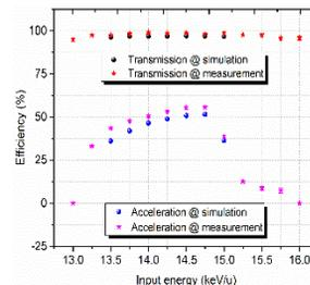
Figure 11: Measured and simulated RFQ transmission and acceleration efficiency versus the input beam energy.
