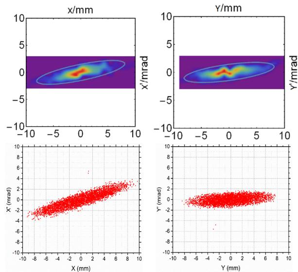
Figure 10: Measured (up) and simulated (down) beam emittance in MEFT test chamber after triplet focusing.
