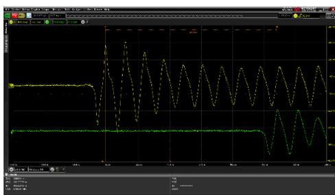
Figure 8: BPM signals (yellow: BMP-1, green: BMP-2).
