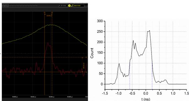
Figure 9: FFC signal (left, red line) and simulated (right) bunch length.
