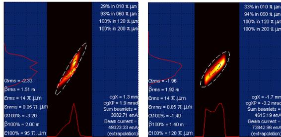
Figure 2: LEBT test chamber 1# emittance measurement for 90 eμA He<sup>+</sup> beam, throttled slits.
