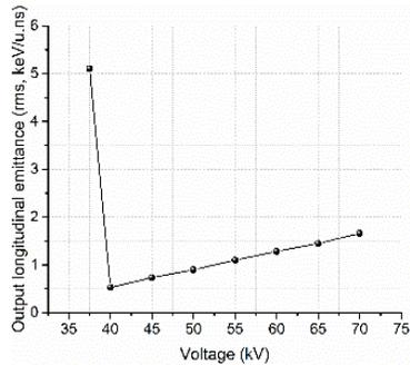
Figure 7: Simulated RFQ output longitudinal emittance as a function of the vane voltage.
