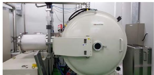
Figure 1: Vacuum furnace for heat treatment: cavity is loaded horizontally.
