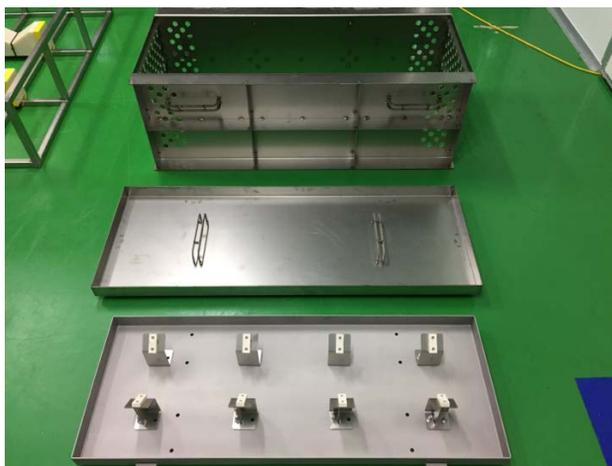
Figure 3: Titanium box: body, top, and bottom part.
