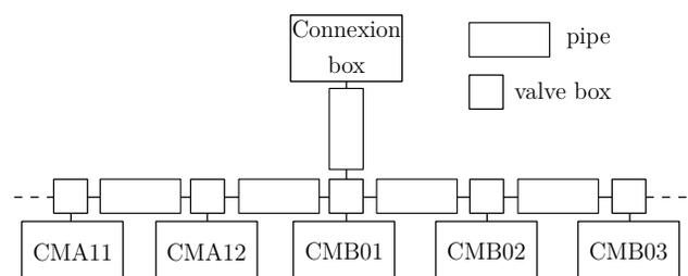
Figure 2: Decomposition of the cryodistribution in multiple pipes -  $CMA_i$  represents type A cryomodule whereas  $CMB_i$  represents type B cryomodule
