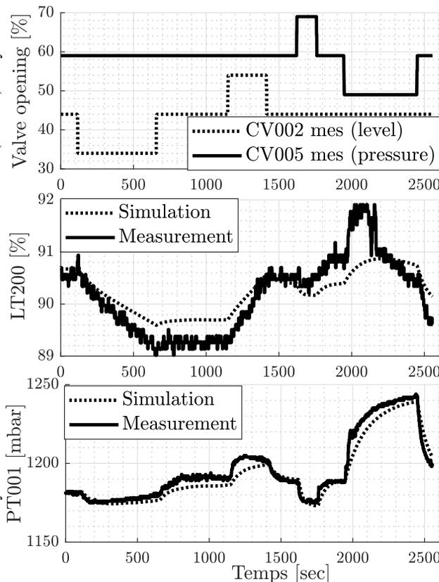
Figure 5: Comparison between experimental and simulated data for type-A cryomodule n°10.
