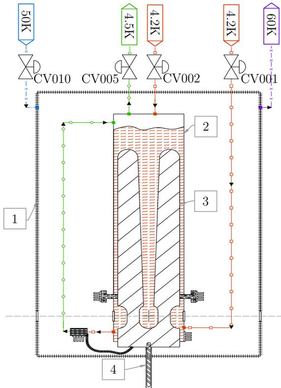
Figure 3: PI& D of type-A cryomodule and its associated valves - 1. The thermal shield, 2. The liquid helium bath, 3. The accelerating cavity, 4. The RF antenna.
