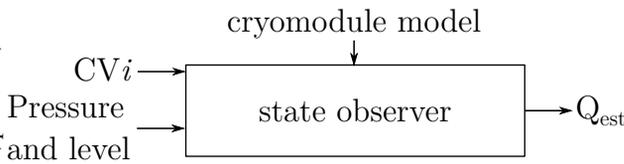
Figure 4: description of the observer -  $CV_i$  represents the valves opening whereas  $Q_{est}$  is the estimation of the dynamic heat load.
