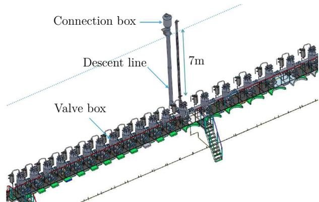
Figure 1: View of the SPIRAL2 cryodistribution without the cryomodules.
