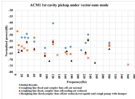
Figure 6: Noise spectra from the phase signal as a function of ACM1 vibration damping. After fixing the roughing bellows and turn off cooling fans most noise peaks are reduced especially the 120 Hz peak; After the cooling air flow is reduced, the noise peaks continue to be reduced with only 3 noise peaks higher than -60 dB; Further damping of the waveguide and the addition of a roughing pump damping pad, the 232 Hz noise peak reduced about -10 dB.
