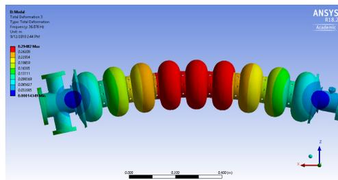
Figure 5: the simulation of 35Hz mode of cavity.
