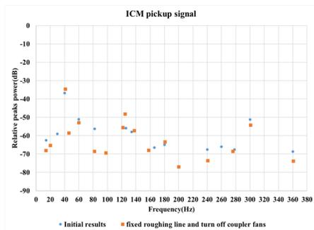
Figure 7: ICM vibration damping.
