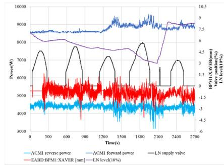
Figure 9: The beam test results with LN<sub>2</sub> supply valve regulated at 120 K. There was still some fluctuation on RF power (forward power in blue and reverse power in green) which became more significant after few LN<sub>2</sub> supply valve opening period (LN<sub>2</sub> level in violet and LN<sub>2</sub> supply valve position in black). The beam energy (red line) had disturbance which correlated with LN valve status.
