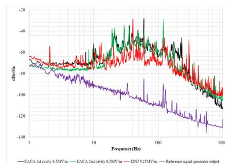
Figure 2: pickup signals noise analyses. During the test the ACM1 was setup in single cavity mode with closed amplitude and phase loop with low proportional gain; the ICM was under operational mode.
