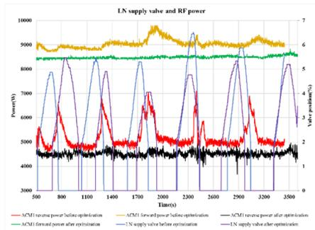
Figure 8: The RF power fluctuation with LN<sub>2</sub> supply valve. The initial regulated temperature was 130K and the reverse power showed 2 kW fluctuation (forward power in yellow and reverse power in red). Then the ACM1 LN<sub>2</sub> regulated temperature decreased to 120 K and the LLRF parameters were optimized, the RF power fluctuation has been reduced (forward power in green and reverse power in black).
