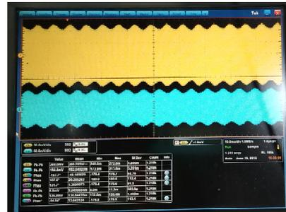
Figure 1: The ponderomotive oscillation of ACM1 pickup signals. The yellow waveform is 1<sup>st</sup> cavity pickup signal and the green waveform is 2<sup>nd</sup> cavity pickup signal.
