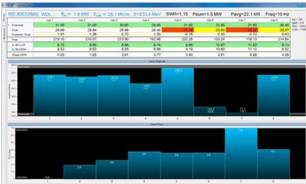
Figure 8: Measuring results of coupling ratio and phase for each output at HPRF test stand.
