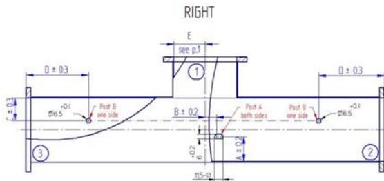
Figure 3: Layout of a right type shunt tee.
