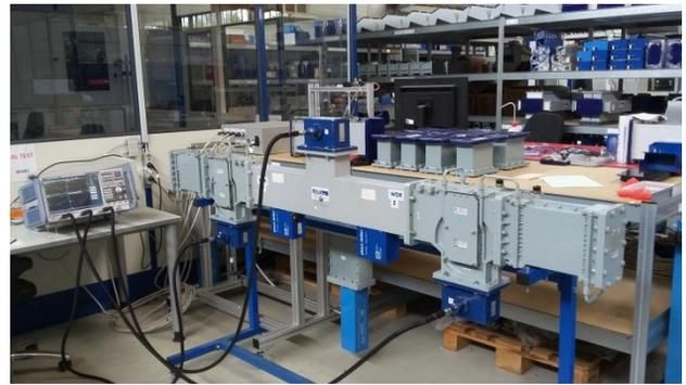
Figure 4: Measuring of a binary cell with all components at the binary cell test stand.
