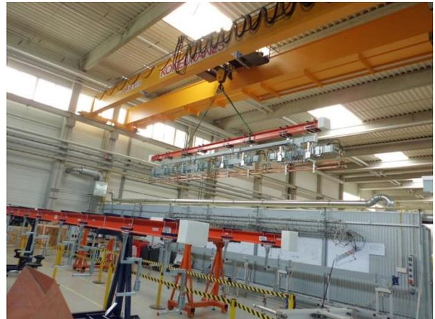
Figure 10: Transportation of the waveguide distribution from WATF to AMTF for installation to the cryomodule.
