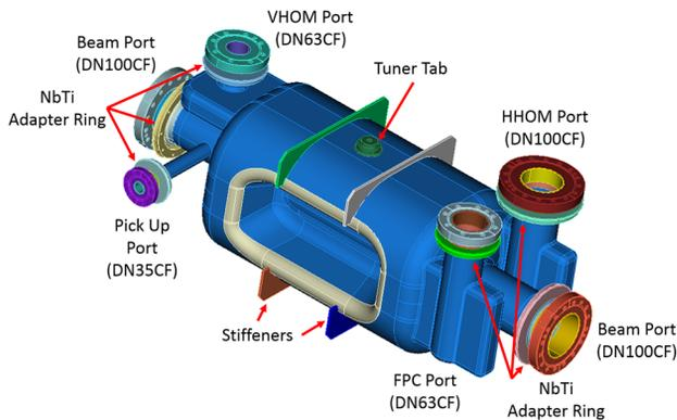
Figure 1: 400 MHz SPS prototype rf-dipole cavity.
