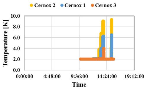
Figure 9: Measured temperature change in Cernox sensors.
