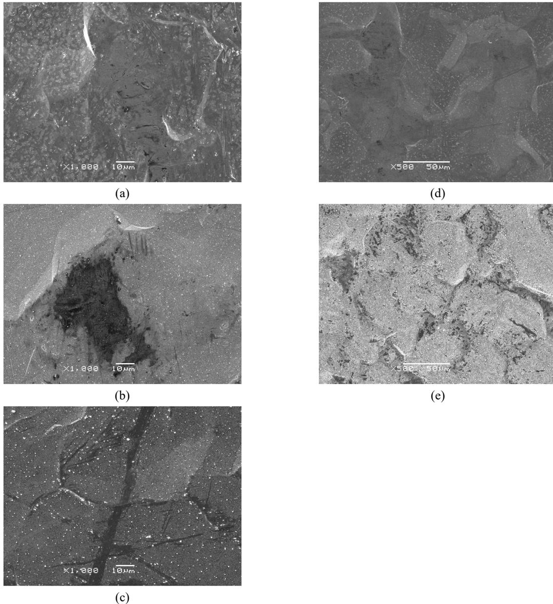
Figure 5: Less-nuclear zones in Nb nucleation samples with SnCl<sub>2</sub> dosage of 11.9mg (a) and 100mg (b). Less-nuclear zones at scratches (c), grain boundaries (e) and even some whole grain surfaces (d).
