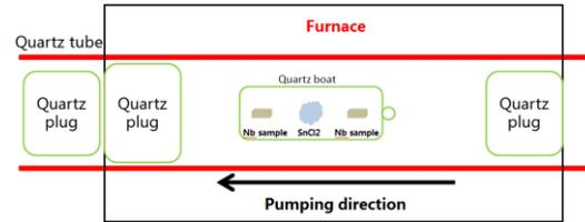
Figure 3: Detailed setup of the experiment to verify the effects of aeration condition.
