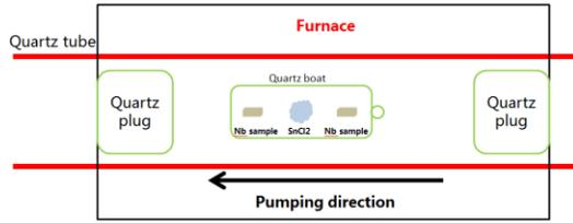
Figure 1: Detailed setup of the experiment to verify the effects of pumping direction.
