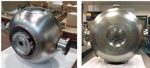
Figure 1: Bare cavity (left) and jacketed cavity (right) of SSR1 prototype.
