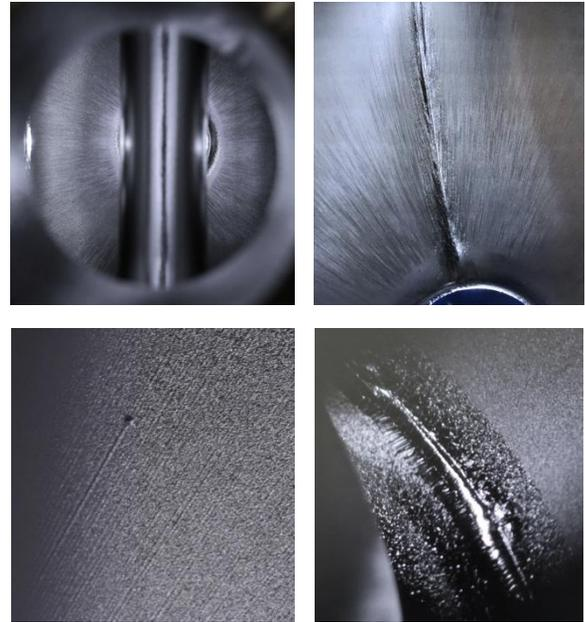
Figure 3: Uneven finish and defects on the RF surface.
