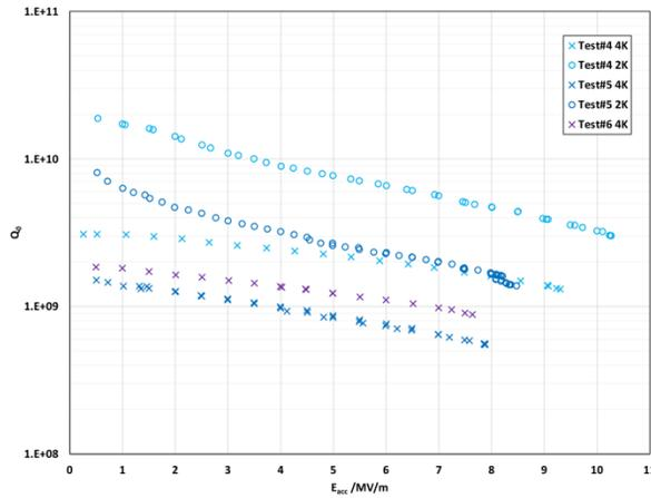
Figure 2: 4K and 2K  $Q$ - $E_{\text{acc}}$  curves of the prototype SSR1.
