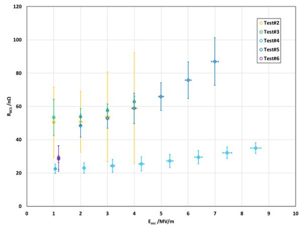
Figure 4: Extracted BCS component of the surface resistance of each cold test at 4K as a function of  $E_{\text{acc}}$ .
