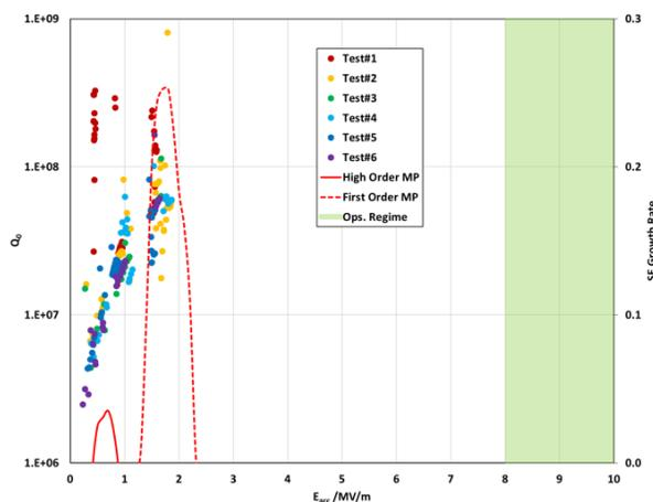
Figure 5: Comparison of measured ( $Q_0$ ) and predicted (secondary electron growth rate) multipacting barriers of SSR1 prototype.
