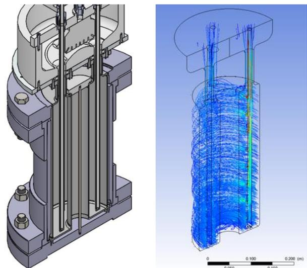
Figure 2: The chemical etching fixture of HWR (left) and the simulated velocity distribution of the acid circulation during BCP process (right).
