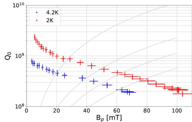
Figure 5: 4 K and 2 K  $Q_0 - B_p$  curves of the fundamental mode of HWR baseline test with the constant power lines at 1 W, 5 W, 10 W, and 20 W.
