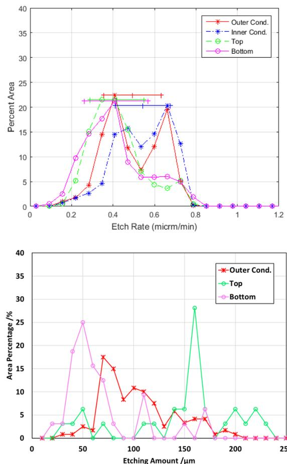
Figure 3: The histogram of the simulated etching rate (top) and the measured etching amount after 120  $\mu\text{m}$  BCP (bottom) of HWR. Various colours represent different parts of cavity.
