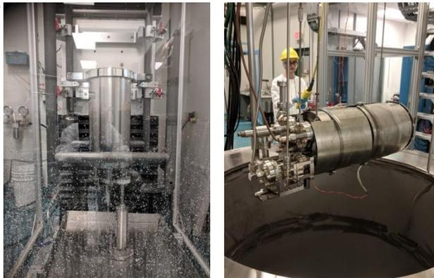
Figure 4: HPR of HWR on the vertical rinsing stand (left) and the hermetic assembly of HWR (right).
