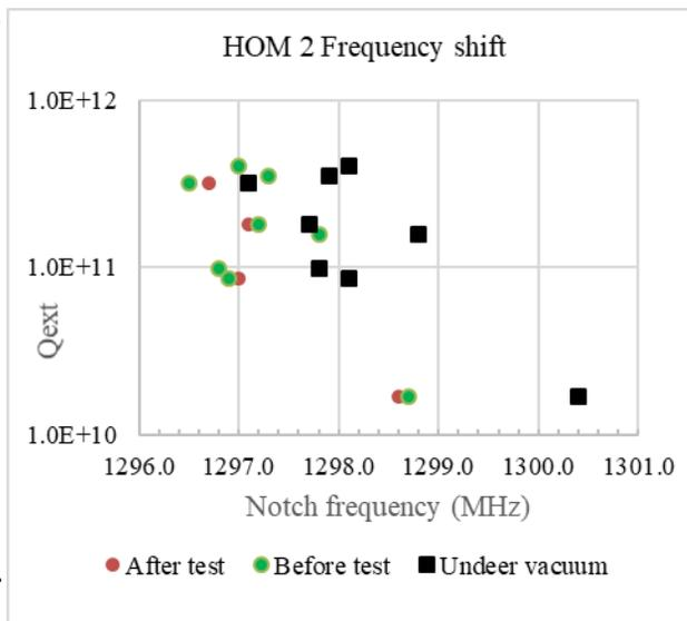
Figure 4: HOM 2 new notch frequency target 1296.3 MHz.
