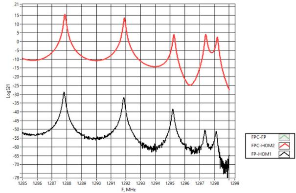
Figure 7: Examples of HOM spectrum: top – properly tuned; bottom – not tuned.
