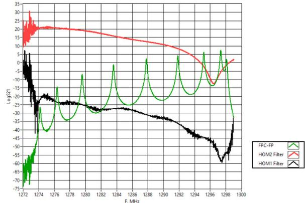
Figure 2: Notch filter view of an LCLS-II cavity spectrum.
