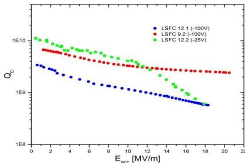
Figure 6: Quality Factor of HiPIMS Nb/Cu LSF cavities ( $B_{\text{peak}}/E_{\text{acc}}=3.68$ ). No field emission was detected.
