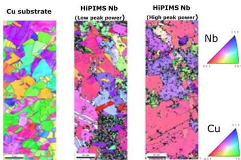
Figure 2: EBSD scans performed on Cu and Nb/Cu samples. From left to right: (a) an uncoated Cu substrate, (b) low peak-power Nb/Cu sample, and (c) high peak-power Nb/Cu sample. OIM color maps included on right for reference of crystal phases.
