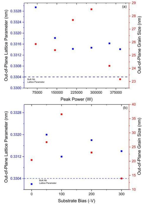
Figure 3: Plot of lattice parameter and grain size vs. (a) peak power in Nb/Cu power series and (b) applied bias in Nb/Cu bias series.
