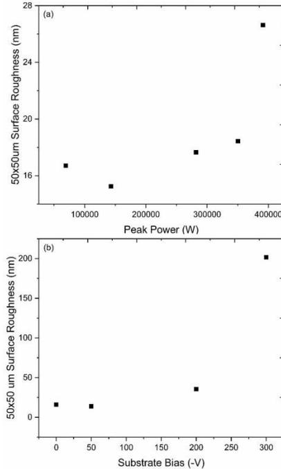
Figure 4: Plot of RMS roughness, on 50×50 μm scale, vs (a) peak power for Nb/Cu power series samples, and (b) applied bias for Nb/Cu bias series samples. Note the roughness scale difference compared to the power series results above.
