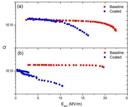
Figure 5: Quality Factor of Nb/Nb coatings ( $B_{\text{peak}}/E_{\text{acc}}=4.19$ ) before (red) and after (blue) coating for (a) the first and (b) the second coating done at JLab.
