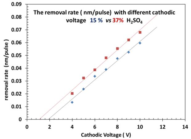
Figure 3: The average removal per pulse increases with cathodic voltage for 15% and 37% H<sub>2</sub>SO<sub>4</sub>.
