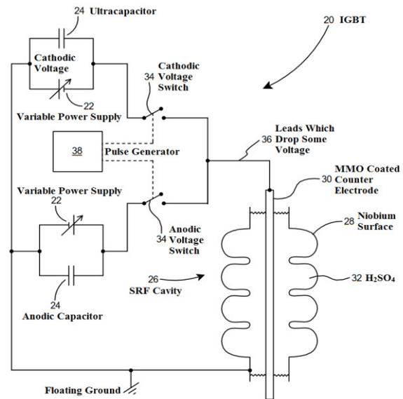
Figure 1: Schematic of the JLab BPEP equipment. [8]
