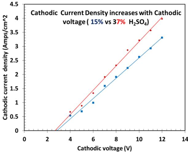
Figure 2: The cathodic current density increases with cathodic voltage for 15% and 37% H<sub>2</sub>SO<sub>4</sub>.
