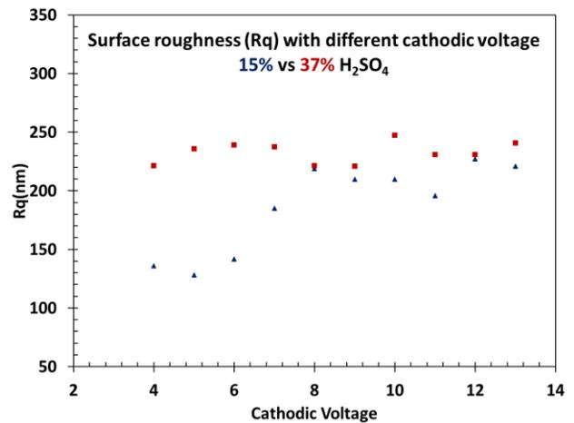
Figure 4: The surface roughness of samples processed by different cathodic voltage for 15% and 37% H<sub>2</sub>SO<sub>4</sub>.
