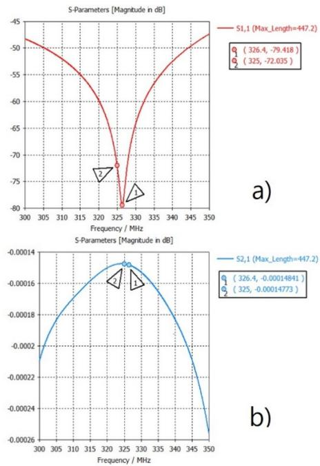
Figure 7: a) Reflected power ( $S_{11}$ ) b) Transmitted power ( $S_{21}$ ) of the power coupler.
