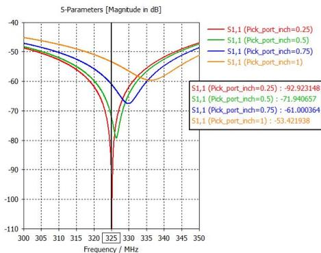
Figure 6: Reflected power ( $S_{11}$ ) change due to diameter change of pick-up port.
