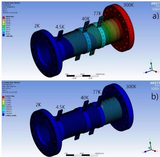
Figure 9: a) Temperature distribution and b) Heat flux result of static thermal load.
