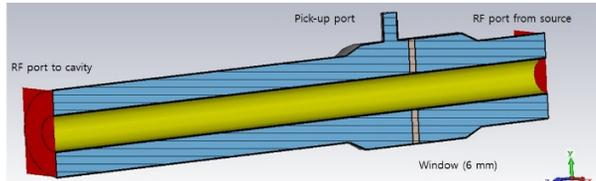
Figure 5: Electromagnetic model of the power coupler.
