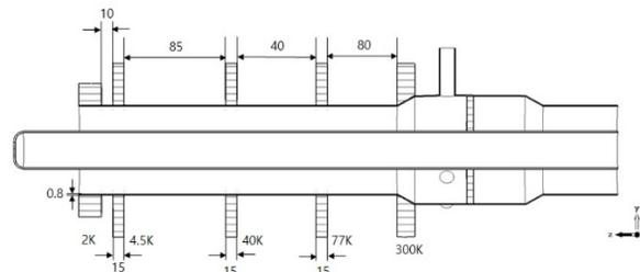
Figure 8: Scheme of a prototype power coupler for thermal analyses.
