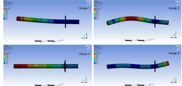
Figure 11: Four resonance modes of antenna.
