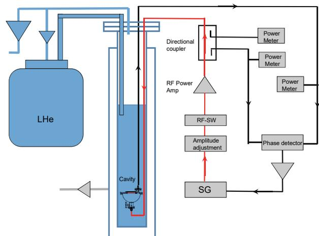
Figure 7: Vertical test setup of mushroom-shaped cavity.
