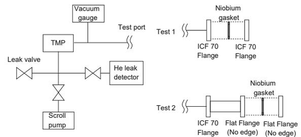
Figure 5: Leak test setup of Nb gasket and flat flange.
