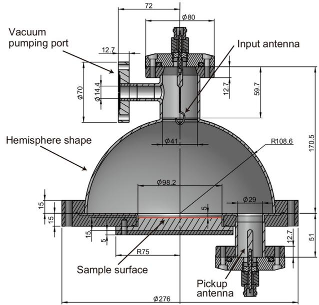
Figure 4: Cross sectional drawing of Nb-based mushroom-shaped cavity.
