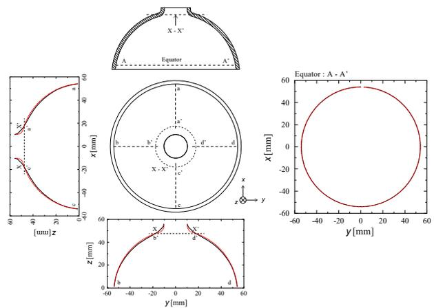
Figure 6: Comparison of press forming shape between design and 3D measurement. Red line is designed line, black line is 3D measurement.
