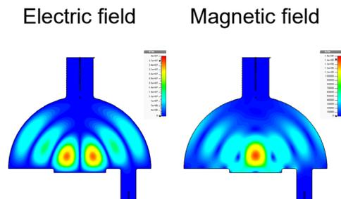
Figure 1: Calculated electromagnetic field in the mushroom-shaped cavity.
