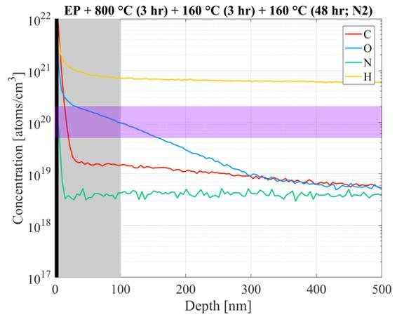
Figure 3: Results of SIMS analysis for a witness sample baked with the 1.3 GHz and 2.6 GHz cavities treated with the 48 hr 160 °C dope. The black line indicates the 5 nm oxide layer at the surface, the gray bar indicates the approximate RF penetration region of 100 nm, and the purple bar indicates the typical nitrogen concentration of a 2/6-doped cavity.
