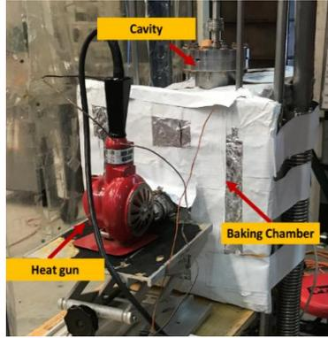
Figure 3: Set-up of 75C baking on the wave-guide insert.
