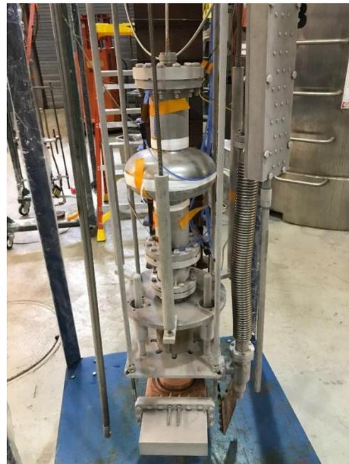
Figure 1: Test insert with single-cell cavity and instrumentation.
