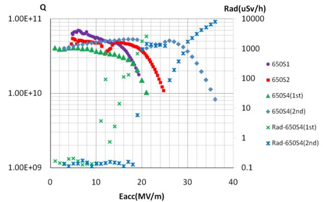
Figure 7: Vertical test results of 650 MHz 1-cell cavities.
