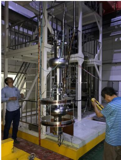
Figure 6: Vertical test of 650 MHz 1-cell cavities.
