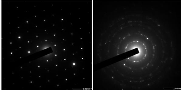
Figure 5: Diffraction patterns of TEM (left: pure Nb; right: Nb N-doped).
