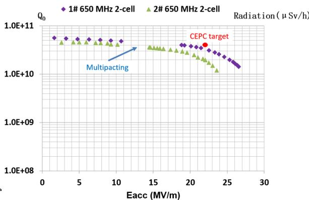
Figure 10: Vertical test results of 650 MHz 2-cell cavities.
