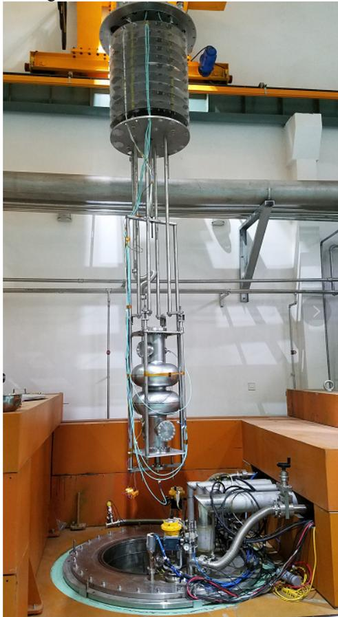
Figure 9: Vertical test of 650 MHz 2-cell cavity.
