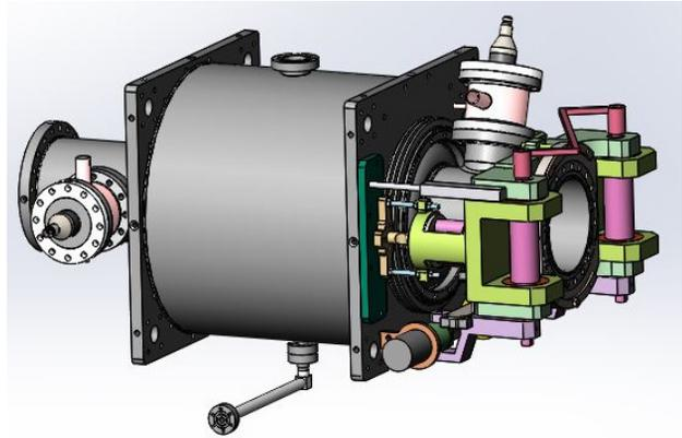
Figure 11: 650 MHz 2-cell cavity with Helium vessel and tuner.
