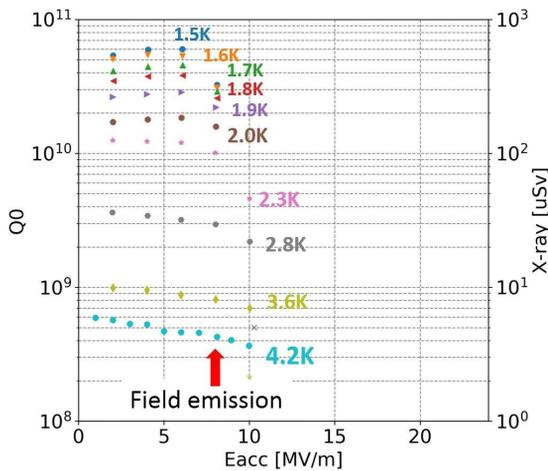
Figure 5: The quality factor measurement retrieved at each temperature from 1.5 K to 4.2 K.
