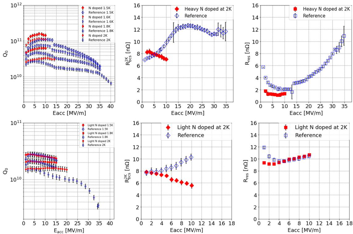
Figure 4: Upper figure shows the result of the heavy doped single-cell cavity. Lower figure shows the result of the light doped three-cell cavity.
