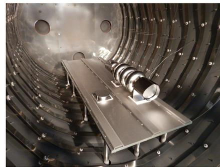
Figure 1: The set-up of nitrogen doping using oil-free furnace at J-PARC.
