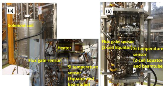
Figure 3: The picture of the set-up for vertical test. a) Solenoid coil, Si sensors and flux gate sensor for single-cell cavity applied heavy dope. Using solenoid coil for cancel ambient magnetic field. b) For three-cell cavity applied light dope without solenoid coil.
