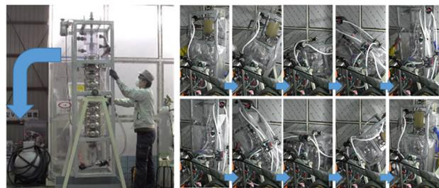
Figure 1: Cavity flip upside down setup and procedure.
