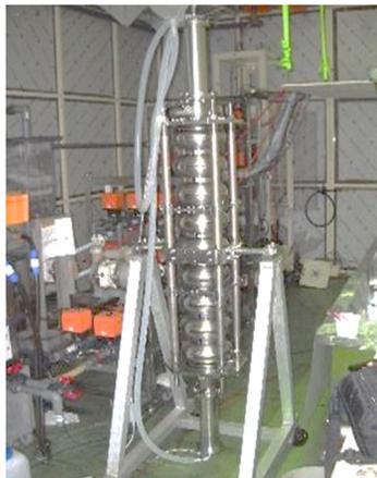
Figure 5: A photo of ultrasonic rinsing process.
