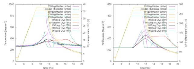
Figure 7: Temperatures of (left) 15K and (right) 80K cryo-panel during operations.
