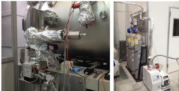
Figure 5: (left) TMP used during Nitrogen-injection. (right) Nitrogen-injection system.
