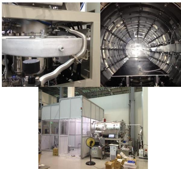
Figure 2: (top left) Water-cooled baffle, gate-valve and cryopump. (top right) Inside furnace. (bottom) Completed furnace with clean booth.
