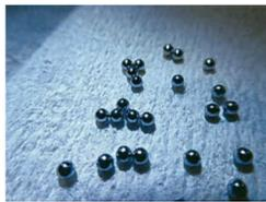
Figure 7: Niobium samples for SQUID.
