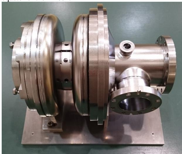
Figure 4: Fabrication completed SRF gun #2.
