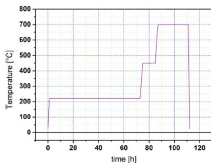
Figure 3: Temperature profile during Nb/Cu/Sn/Cu solid diffusion.
