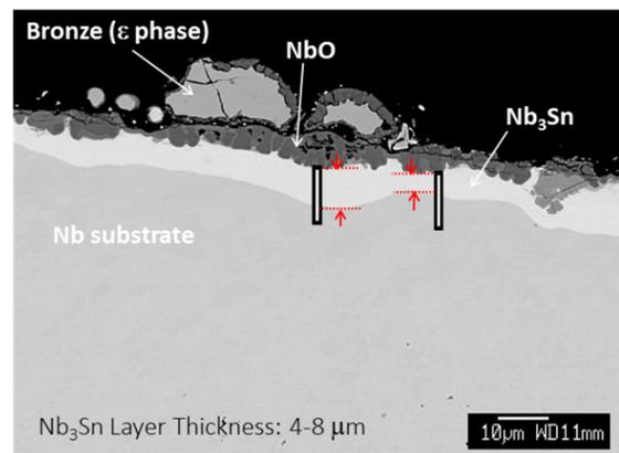
Figure 4: Cross-section of a sample with EPMA results (NIMS).
