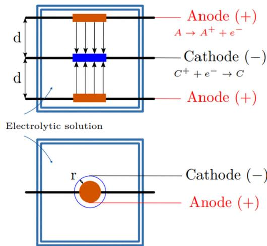
Figure 1: Schematic of electro-chemical cell for bilateral coating of Nb flat samples (top), and internal coating of Nb cylinders (bottom).
