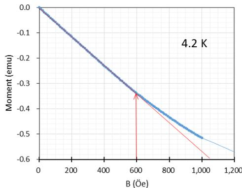
Figure 7:  $M$ - $H$  curve obtained with SQUID magnetometer at NIMS. The  $H_{c1}(4.2\text{K}) = 600$  Oe.
