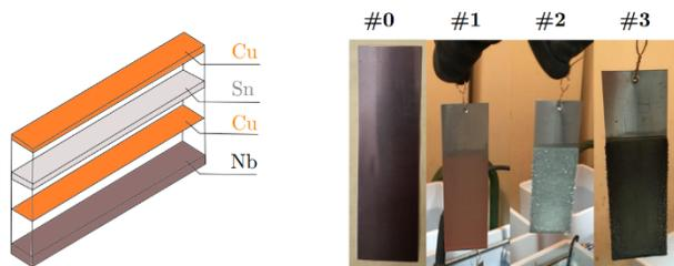
Figure 2: Sequence of deposited layers (left), and pictures of sample at each deposition step (right).
