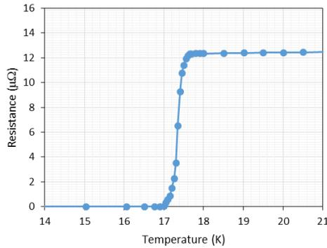
Figure 5: DC test at FNAL of  $T_{c0} = 17.5$  K of a  $\text{Nb}_3\text{Sn}$  film sample.
