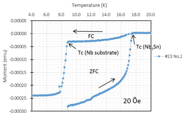
Figure 6:  $M$ - $T$  curve obtained with SQUID magnetometer at NIMS. The  $T_{c0} = 17.6$  K.
