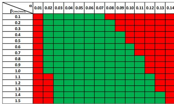
Figure 4: This Matrix provides an overview over the combinations of the initial Twiss parameters  $\alpha_{in}$  and  $\beta_{in}$ , that did (green) and did not (red) lead to what were considered to be exit beams of sufficiently high quality.
