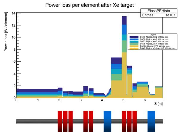
Figure 5: BDSIM halo tracking simulation with aluminium beam pipes of different diameters. The most power is deposited after the first dipole magnet.
