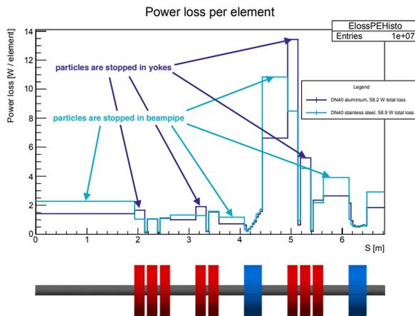
Figure 4: BDSIM halo tracking simulation with DN40 aluminium and stainless steel beam pipes. Drift sections are gray in the lattice plot, quadrupoles red and dipoles blue.
