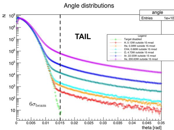
Figure 2: Geant4 simulation of the angle distributions with and without a gas targets as designed for MAGIX. All target gases are modeled with a particle density of  $10^{19} \text{ cm}^{-2}$  and the beam current is assumed to be 1 mA. TAIL region starts at 15 mrad, corresponding to  $6\sigma_{\text{beam}}$ .
