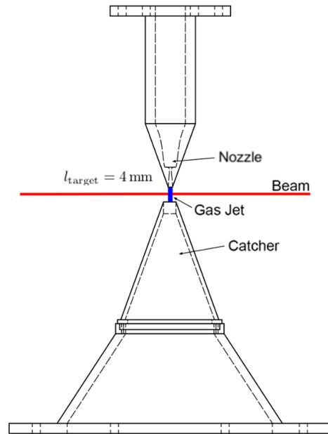
Figure 1: Schematic drawing of the MAGIX gas target [5].
