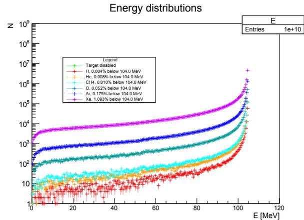
Figure 3: Electron energy spectrum after target passage. Beam mean energy remains virtually untouched, while few low energy particles are produced through scattering.
