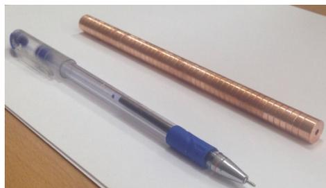
Figure 11: Brazed W-band structure.
