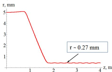
Figure 9: Beam envelope in the field of permanent magnets.
