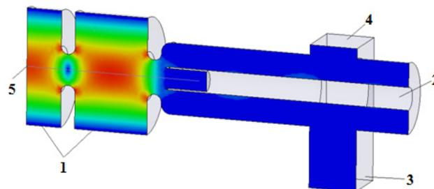
Figure 1: Layout of the photocathode gun with the electric field distribution: 1 — accelerating cavities, 2 — input for the laser beam, 3 — RF power input, 4 — vacuum pumping connection, 5 — photocathode.
