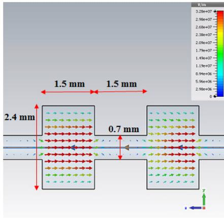
Figure 4: Two cavities of the excited W-band structure by the beam with  $\sigma_t = 2$  ps,  $Q = 2$  nC.
