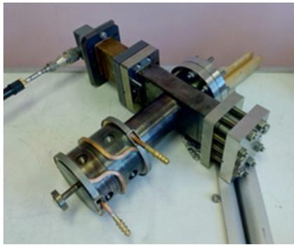
Figure 3: Fabricated photocathode RF gun.
