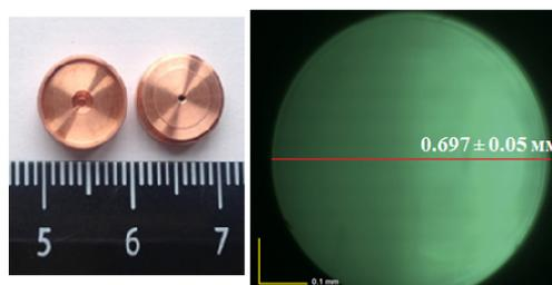
Figure 10: On the left – cavities, on the right – depiction of the aperture obtained with help of microscope.
