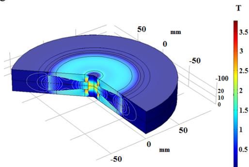
Figure 7: Magnet module with field lines.
