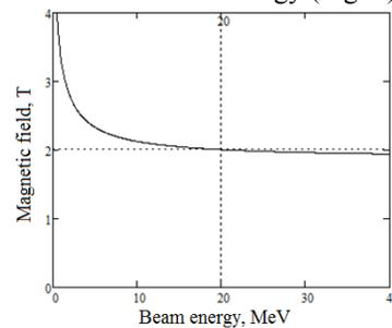
Figure 6: Dependence of focusing magnetic field on the beam energy.
