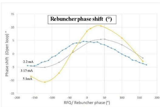
Figure 11: Phase variations, with the phase setting point of the rebuncher, open loop.
