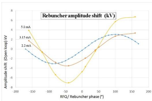
Figure 10: Voltage variations, with the phase setting point of the rebuncher, open loop.
