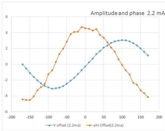
Figure 9: Voltage and phase variations, with the phase setting point of the rebuncher.
