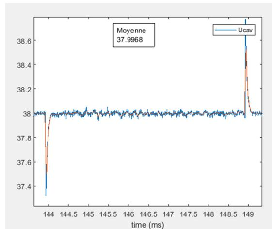
Figure 7: Voltage variation, closed loop.
