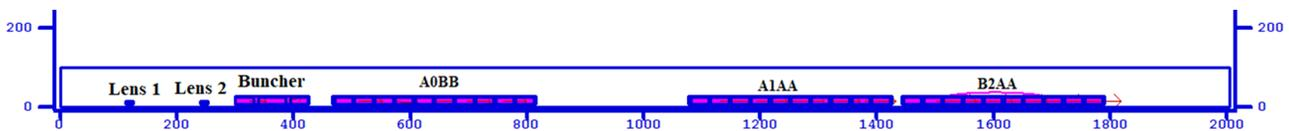
Figure 2: The layout of the magnetic system for accelerating stations A00 – A02 in POISSON program interface (sizes are in cm).
