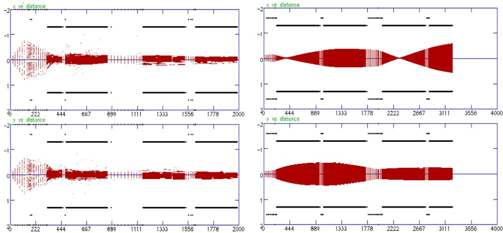
Figure 4: Changes of the transverse dimensions of the beam during acceleration and transport of the beam in accelerating stations A00 – A02 (on the left) and A03 – A04 (on the right).
