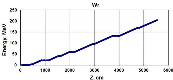
Figure 6: Energy gain along the LINAC-200.
