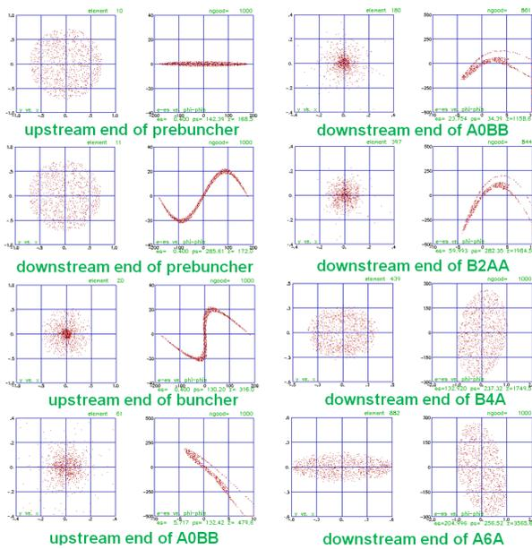
Figure 5: Beam spot (cm), energy-phase distribution (keV, degree).
