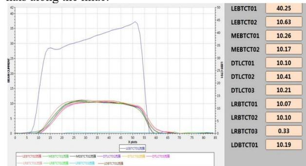
Figure 2: Current Transform Signals of CSNS Linac.
