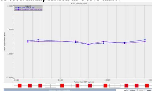
Figure 3: Beam Orbit of MEBT after Orbit Correction.
