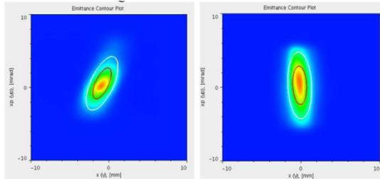
Figure 4: Particle Phase Ellipse by Double slit System: (Left- horizontal, Right-vertical).
