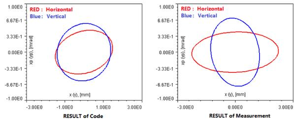
Figure 5: Transverse Phase Ellipse at DTL exit: (Left-simulations, Right-measurement).
