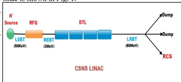
Figure 1: The CSNS Linac Layout.
