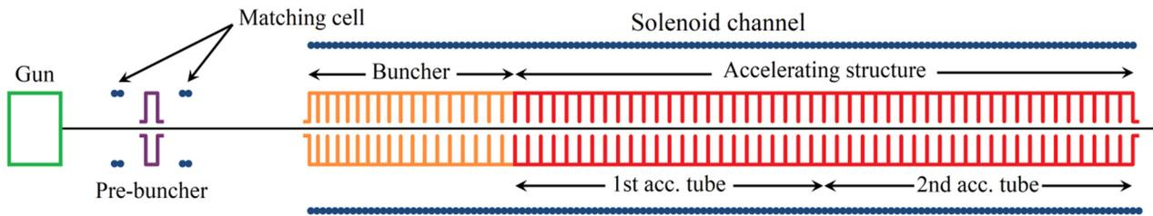
Figure 1: General layout of the ipm linac.
