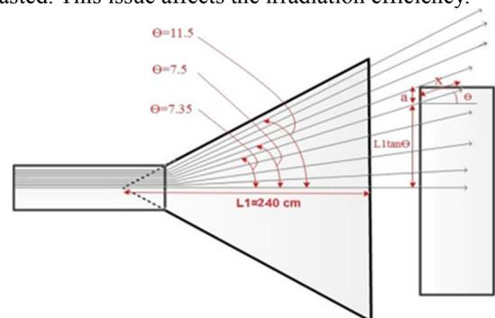
Figure 2: Geometrical parameters at the horn of the beam extraction system.
