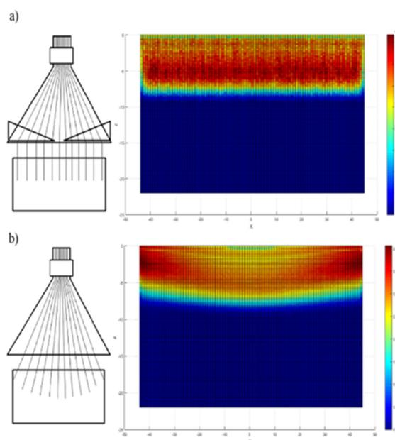
Figure 3: Distribution of doses on the transverse plate. a) perpendicular irradiation. b) divergent irradiation.
