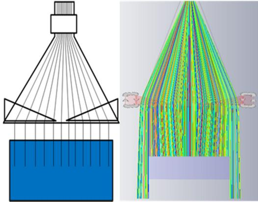
Figure 4: Use of correcting magnets located at the exit window of the horn allows changing the path of the beam.
