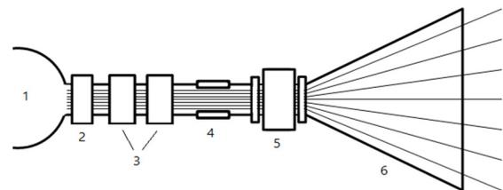
Figure 1: Components of extraction system and transmission of output beam of Linac accelerator. 1) accelerating structure, 2) control magnet, 3) quadrupole doublet, 4) diaphragm, 5) scanning electromagnet, 6) horn.
